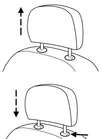
3. Lower the head restraint by pressing and holding the guide sleeve lock/release button and pushing down on the head restraint.
